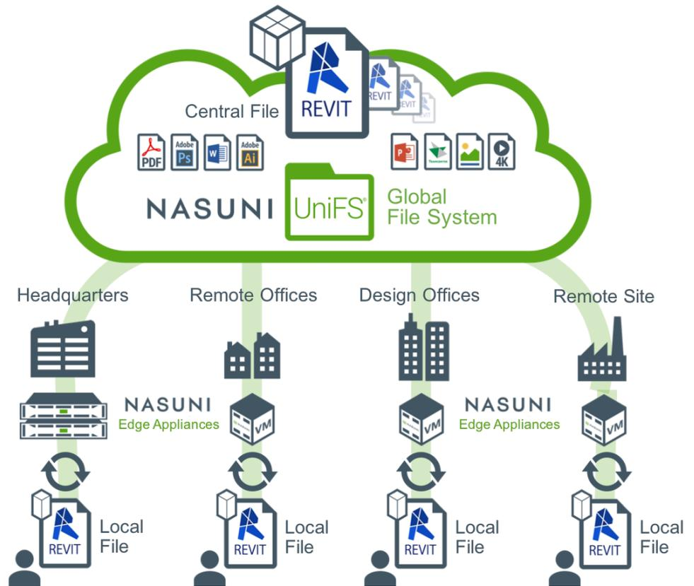
*Nasuni naturally synchronizes changes made to the cached copies of Revit models in multiple locations with the central Revit model in private or public cloud object storage, keeping an immutable version history of all changes.*
